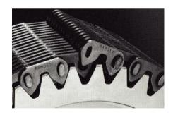
Symmetric chain lacing during connection
